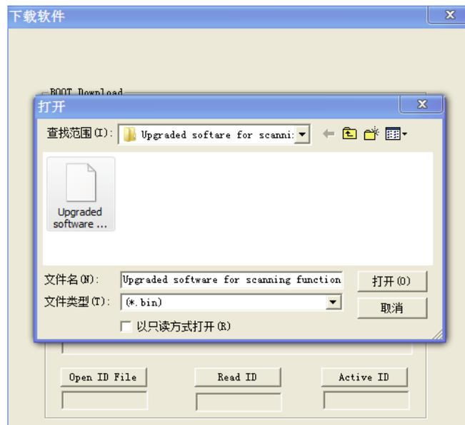
3. Once the new firmware file has been selected and the radio is connected to the PC using the programming cable, click the "Download Update File" button and the firmware will be updated.
